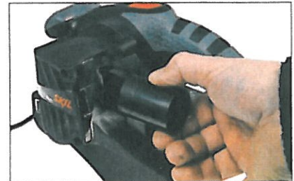
The box can be replaced by a connector for a vacuum hose
