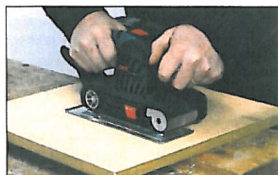
The frame allows safe sanding of veneered boards
