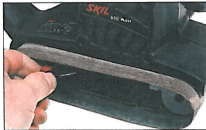
The belt is removed by slackening off the tension lever
